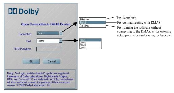
Figure 3-1 Open Device Screen
