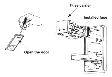
Figure 2-2 Checking the Main Fuse
