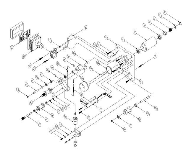
Figure B-13: Central Pivot Analog Soundhead Assembly (196260-001)
