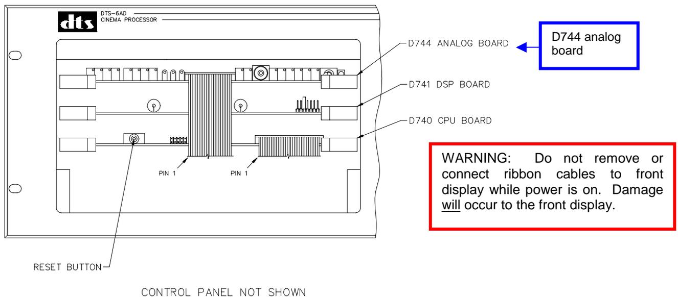
3. Visually inspect the old D744 board for the type of crossovers installed in your CP and verify that these are correct for your installation.
