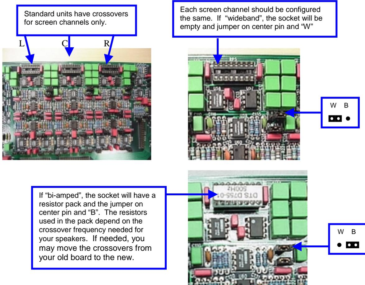
4. Once you have verified that the new board has the correct crossovers and all it's jumpers are set, install the new D744 board
