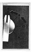
Advance motor switch counterclockwise to position, after motor starts, advance to R(Reverse).
