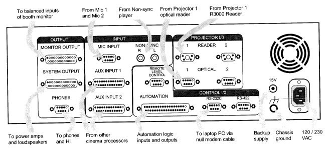
Note that these D-Sub connectors have metric  $(M2.5 \times .45)$  jack screw receptacles and require mating connectors with metric jack screws. A kit of such connectors is provided with each DFP D3000. **Do not use standard D-Sub connectors with 4-40 jack screws.**
