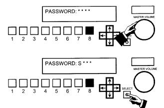
**5.3.9** When you enter the last correct character you will see the ADMIT option flashing. Press the SE-LECT button to proceed to the A-Chain functions menus.
