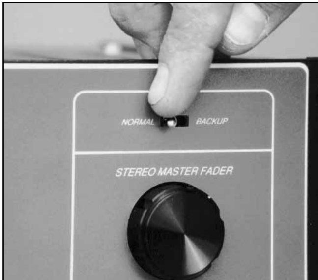
The Normal/Backup switch and Stereo Master Fader
