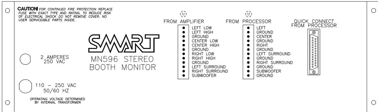
**Connections.** The MN596 has Phoenix connector inputs for amplifier and processor signals, as well as an alternate THX standard DB25 processor connection (see diagram at right). Simply connect appropriate amplifier and processor signals to the indicated Phoenix positions.
