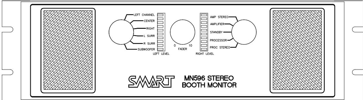
**Listening Modes.** The right knob controls listening mode. When set to AMP STEREO or PROC STEREO, the MN596 sends Left and Center channel signals to the left speaker, and Right and Center channel signals to the right speaker, creating a stereo sound with a “phantom” center channel. The left knob selects the individual channel monitored in the AMPLIFIER and PROCESSOR listening modes. STANDBY mode disconnects all monitoring signals, but does not power down the system.
