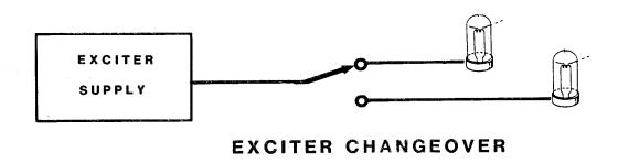
INSTALLATION OF AN EXCITER CHANGEOVER. MAKE SURE THE SWITCH OR AUTOMATION CAN HANDLE 5 AMPERES. THE EX500B EXCITER SUPPLY WILL NOT POWER TWO EXCITER LAMPS AT THE SAME TIME.
