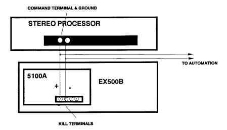
CONNECT THE (+) TERMINAL OF THE "KILL" TERMINAL TO THE "COMMAND" TERMINAL OF A SMART PROCESSOR, AND THE (-) TERMINAL TO A NEARBY GROUND TERMINAL OF THE PROCESSOR. EXTEND THE PAIR OF WIRES TO THE AUTOMATION SYSTEM NON-SYNC CONTROL. THE EXCITER WILL GO TO A PRE-HEAT CONDITION DURING INTERMISSION.
