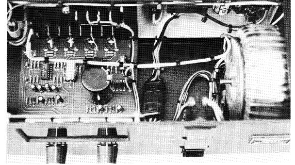
A VIEW OF THE INSIDE OF THE CHASSIS WITH THE TOP COVER REMOVED. NOTICE THE PLUG THAT ALLOWS THE EXCITER SUPPLY MODULE TO BE REMOVED QUICKLY. REMOVE 4 SCREWS ON THE OUTSIDE OF THE 5100A MODULE TO REPLACE THE MODULE.
