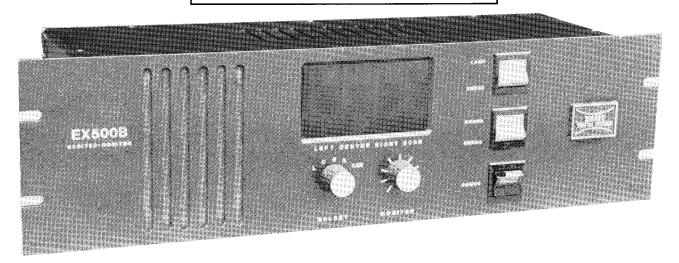
THE EX500B IS A COMBINATION 4-CHANNEL BOOTH MONITOR AND REGULATED EXCITER LAMP SUPPLY IN ONE COMPACT 19" RACK MOUNTED UNIT.
