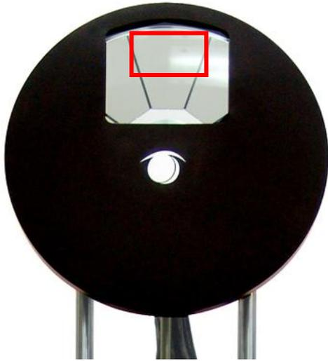
8. Project an image on the screen and “fine adjust” the position of the image on the MI-2100 filter – The image should be just below the top of the filter area and equally spaced on the left and right sides.
