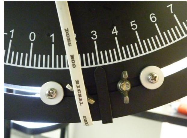
10. Insure the sensor indicator on the bottom of the MI-2100 filter cover is set to the number 3, and it is tightly secured.
