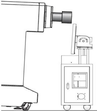
1. Position the MI-2100 in front of Projector and determine the best orientation based on having the filter close to the lens within the space available in front of the projector. The filter position can be adjusted using the slots in the motor base.
