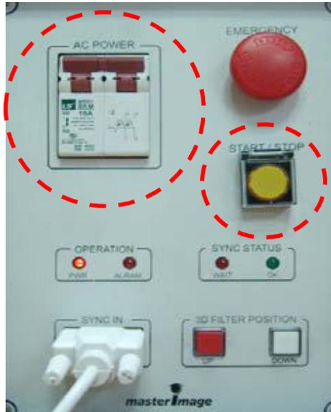
13. With the projector in 3D mode/channel, insure the Main Power breaker is “On” and system is ready to start (Red “PWR” LED and Red “WAIT” LED are on). Push the yellow Start/Stop button.
