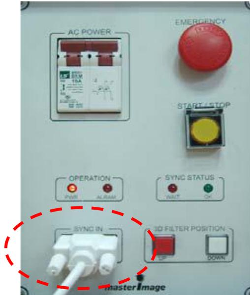
5. With the MI-2100 power breaker in the off position, connect the supplied SYNC Cable to MI-2100 and the GPIO port of the Projector.
