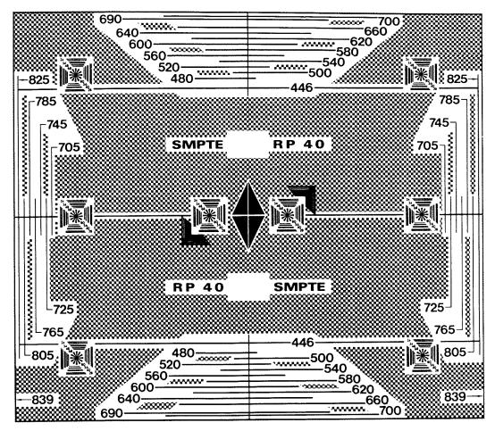
Figure 3. 35 mm Projector Alignment and Image Quality Test Film (SMPTE No. 35-IQ).
