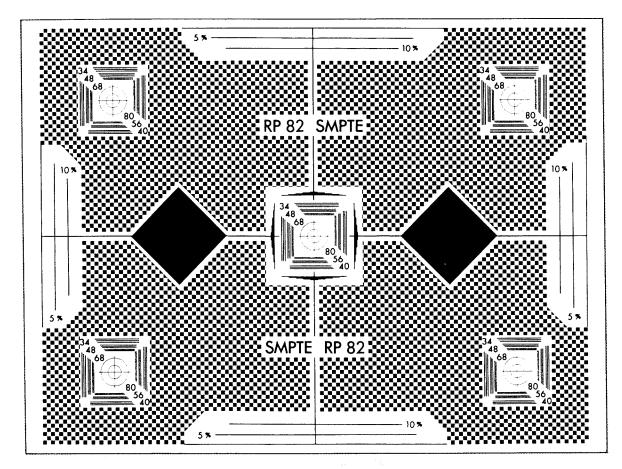
Figure 5. 16 mm Projector Alignment and Image Quality Test Film (SMPTE No. 16-PA-100).
