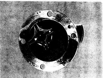
Figure 4. Partially disassembled Geneva movement showing the CAM and PIN mechanism.
