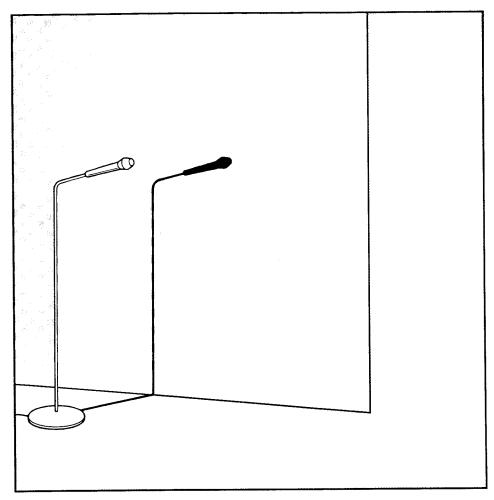
Figure 4. Vertical unsteadiness can be checked easily by observing image movement next to a shadow of some object placed near the screen (see text below).
