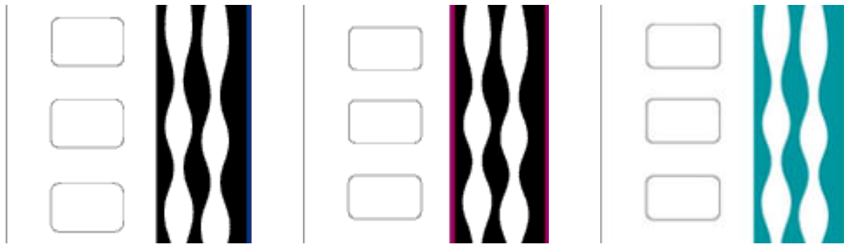
Figure 3. Left to right: Conventional silver-applied soundtrack, silver-applied track with "high magenta" dye layer, and cyan dye-only soundtrack.
