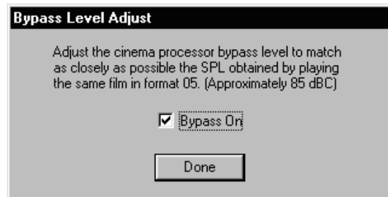
Figure 2-12 Bypass Level Adjust
