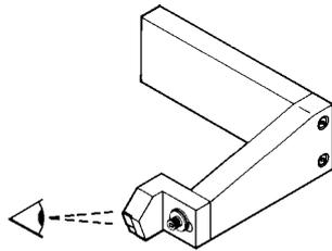
If a stereo solar cell is already installed on Projector No. 1, inspect the surface of the cell for cracks, chipping, or other damage. If the cell appears to require replacement, remove the mounting bracket from the projector and replace the cell and mounting block assembly.
