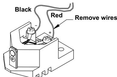
5. Attach the wires to the replacement LED assembly using the same wire locations as in the original LED assembly. The wires may require restripping since they have been compressed previously, and could be too weak. Inspect the wires carefully before attaching them to the terminals.
