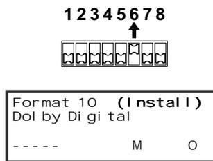
Slide DIP switch-6 to the UP position. This switches the CP650 into setup mode.
