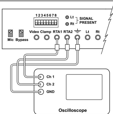
Connect an oscilloscope to the following test points located on the setup panel:
