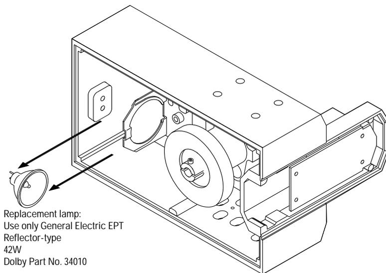
**Figure 9–2 Digital Soundhead Exciter Lamp Replacement.**
