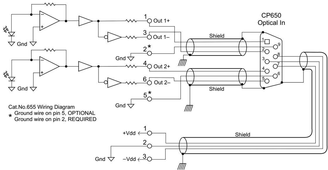
**Figure 2-3 Wiring Using Two 3-Conductor Shielded (screened) Cables**
