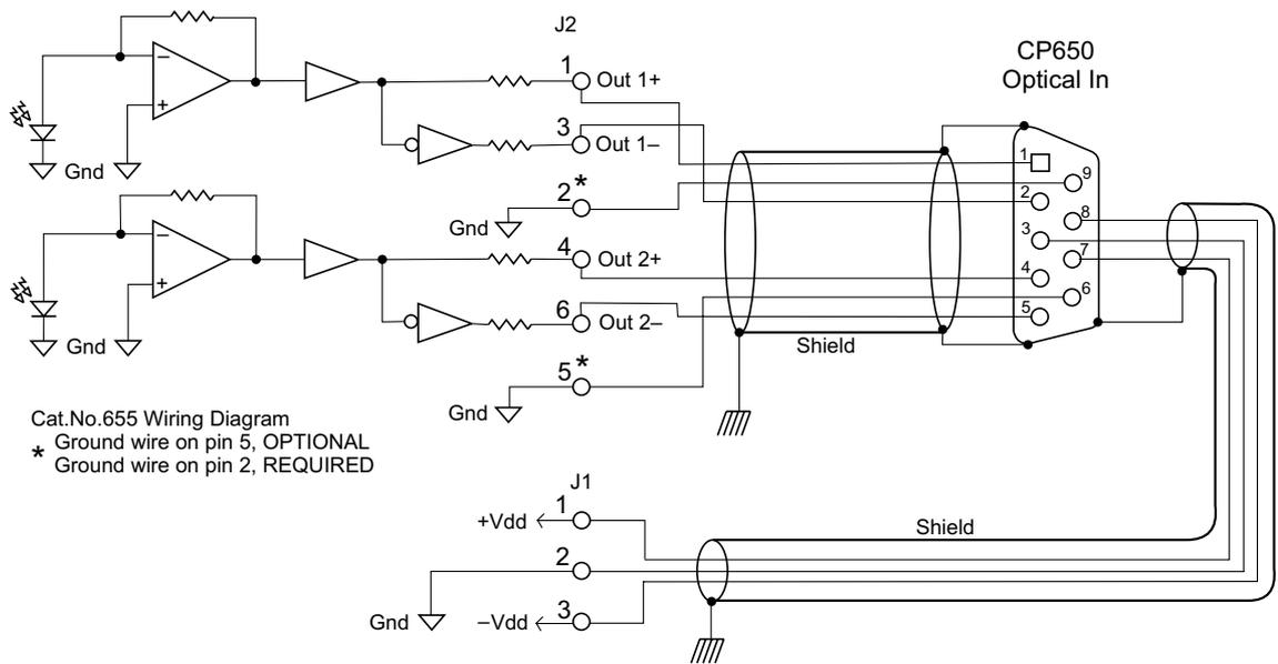
**Figure 2-4 Wiring Using One 5- or 6-Conductor Shielded (screened) Cable**
