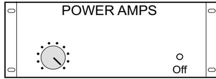
Set all the gain controls on all power amplifiers to a known repeatable setting. **The preferred setting for most amplifier gain controls is maximum.**
