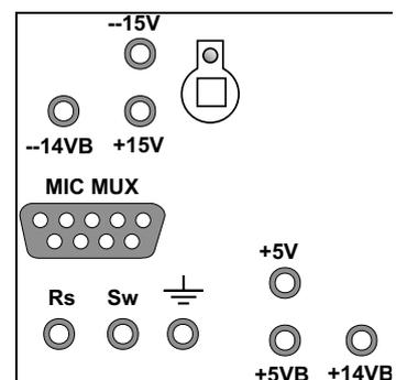
**Figure 3-4 Power Supply Voltage Test Points**
