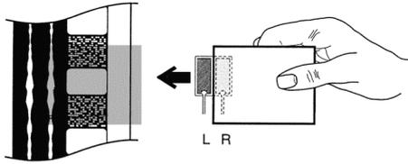
Verify that the outputs of the right and left solar cells are properly connected by placing a white card over the right sound track (nearer the outside of the projector) and verifying that the level of the right channel drops, as indicated by the **Rt Signal Present** LED on the CP650 setup panel.
