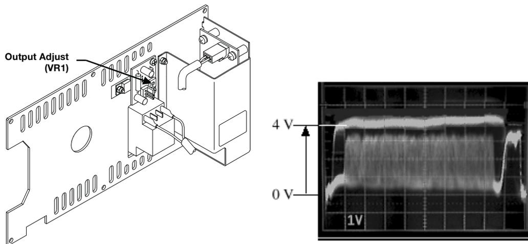
Figure 6–3 Cat. No. 701 LED Brightness Adjustment
