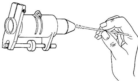
Clean the lens surfaces with a cotton swab moistened with glass cleaner. But keep in mind that you may find, during optical preamp adjustment, that it will be necessary to remove and inspect the lens if the high-frequency response is not correct.
