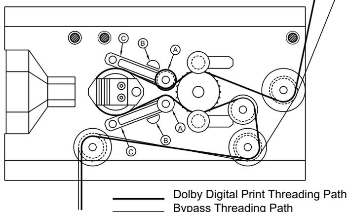
Figure 6-1 Digital Soundhead Adjustments
