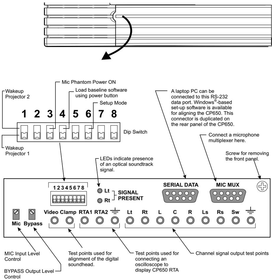
Figure 3-3 Setup Control Panel Description
