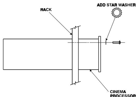
Figure 2-2 Install Star Washers to Rack Mounting Screws
