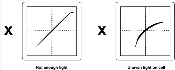
Also, if the ends of the trace display thicker than the center area, then improper lighting of the edges of the optical tracks should be corrected.
