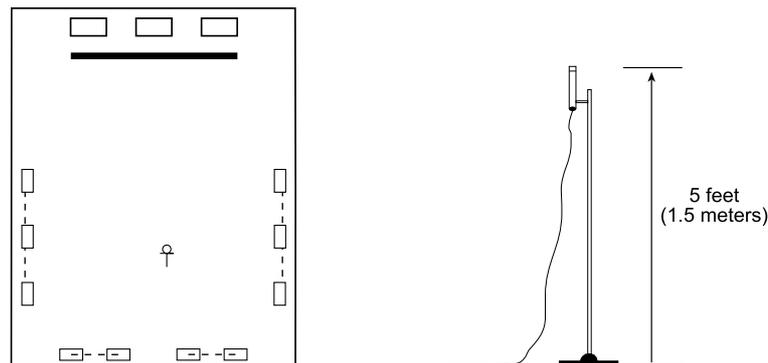
**Figure 4-1 EQ Microphone Placement**
