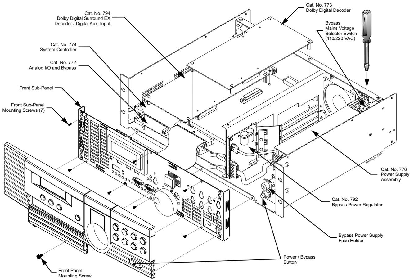
**Figure 2-7 Model CP650 Exploded View**
