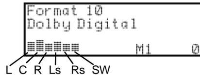
Day-to-day operation of the CP650 is performed through interaction with this display. The 20-character, four-line LCD provides a read-out of processor condition, operation mode, and is used to perform local alignment of the CP650 by the service engineer if PC setup software is not used.
