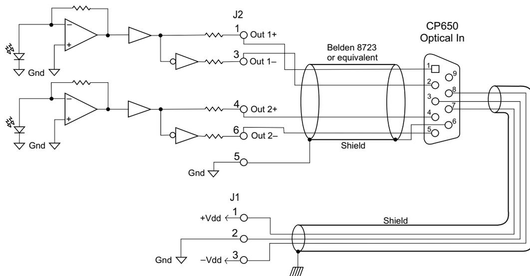
**Figure 2-6 Wiring Using One 4-Conductor Shielded (screened) Cable**
