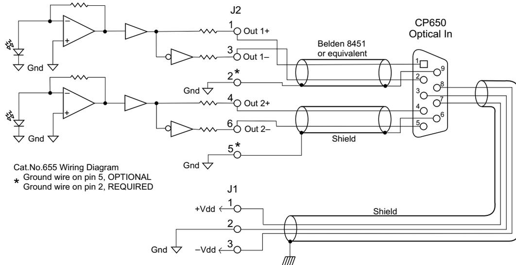
**Figure 2-5 Wiring Using Two 2-Conductor Shielded (screened) Cable**
