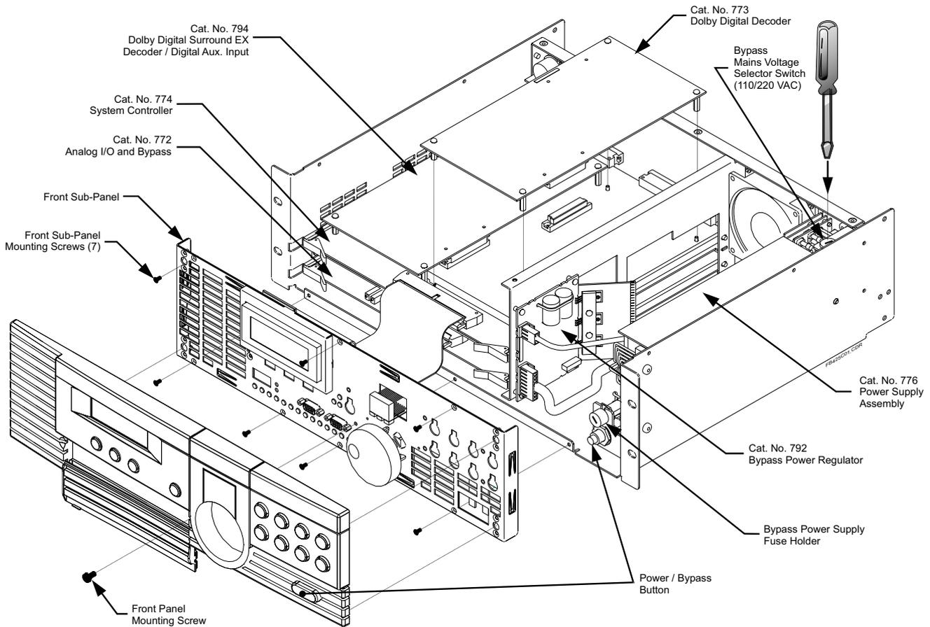
Figure 9–3 Model CP650 Exploded View
