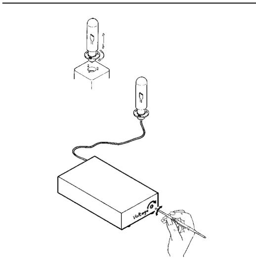
Remove the existing exciter lamp and replace with a new lamp.
