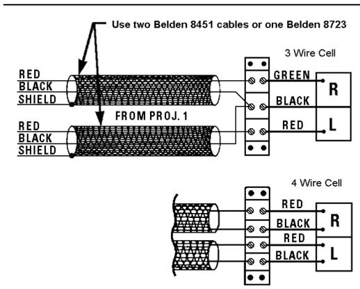
Confirm that the cell wiring and connections are correct. Shielded cables must be used. The inner conductors must be wired to the CP650 OPTICAL input connectors exactly as shown on the wiring diagram foldout.
