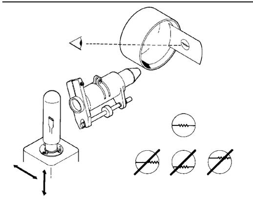
Place a white card at the front of the lens close to the position of the film sound track. Adjust the position of the exciter lamp until the image of the filament is centered both vertically and horizontally as shown.
