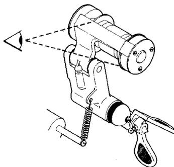
Inspect the lateral film guides for evidence of cuts, cracks, surface defects, or any foreign materials that could impair the film guiding. Clean or replace the guides, as necessary. The guide roller must rotate freely; if it is spring-mounted, make sure that lateral movement and return are not obstructed. If the roller has a felt or rubber insert, check for a flat spot and replace the roller if necessary.
