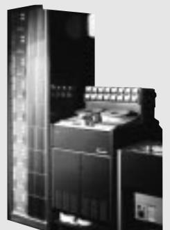
Early multitrack installation with Dolby A301 units.
