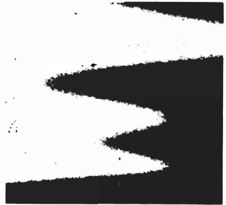
1. A section of optical sound track magnified about 250 times. The granular structure of the track is clearly visible.
