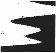
1. A section of optical sound track magnified about 250 times. The granular structure of the track is clearly visible.
