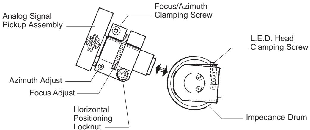
Loosen the focus/azimuth clamping screw and set the focus and azimuth by running the “pink noise” loop and adjusting the signal pickup assembly in the same manner as a conventional slit lens. Finalize the “A” chain installation by again checking the L.E.D. adjustment using Dolby Cat. No. 566 “illumination uniformity” test film. Perform a final “Dolby” level set, and complete any other steps specified by the manufacturer of the sound processor.
