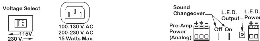
The L.E.D.'s are bipolar; the power supply cannot damage an L.E.D. through reversed polarity. It is safe to try reversing the polarity if you have power but no light. **Accidental connection of the L.E.D. to the pre-amp power terminals will damage the L.E.D.** The pre-amp power to the analog reader (Signal Pick-Up) is 12 V.DC+, ground, and 12 V.DC-. The ground must be connected at both ends as it is circuit reference zero volts.
