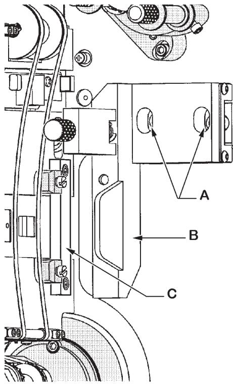
1. Open the turret. Dismount the gate pressure pad runner by loosening the captive thumb screw and removing the runner from the gate carriage.
