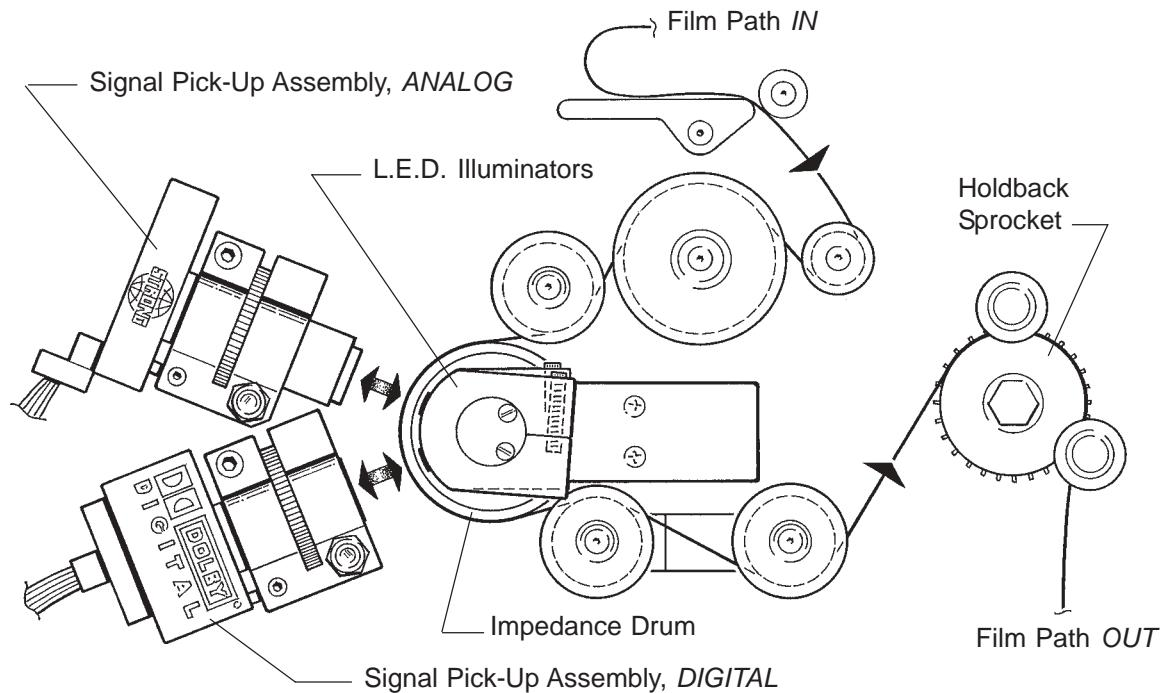
The duty cycle (time ON) of the L.E.D. is the same as the projector motor and should parallel that of the xenon bulb; the lamphouse elapsed hour meter should indicate approximate L.E.D. hours. L.E.D. manufacturers have noted a 10-20% drop in light output after prolonged operation. If a sound signal loss cannot be corrected by fader gain, it may be necessary to replace the L.E.D. head.
