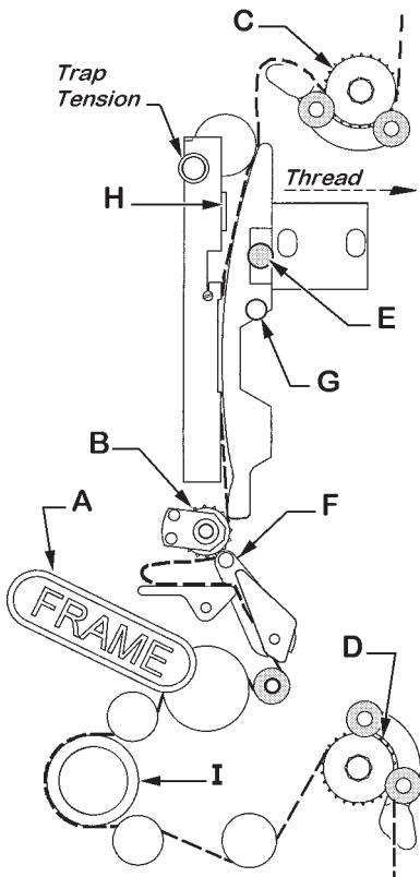
Unlatch and open the turret. Rotate the framing handle (A) to position the intermittent sprocket (B) at the center of its adjustment range. Using the motor flywheel, turn the mechanism by hand to rotate the intermittent sprocket (B) to its "rest" position. In the "rest" position, the intermittent sprocket is in a locked, stationary stage while the other sprockets continue to rotate.
