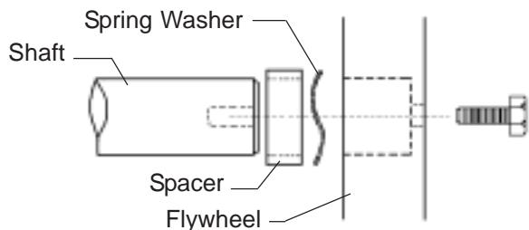
The sound reader flywheel is dismounted for shipping to avoid damage to the impedance drum shaft. Assemble the flywheel to the end of the impedance drum shaft using the wave spring washer and spacer in the sequence shown (spring washer against the flywheel, spacer next to bearing seal). Secure the flywheel to the shaft with the 1/4 inch hex head screw. Note *LEFT-HAND THREAD*; turn *councclockwise* to tighten.
