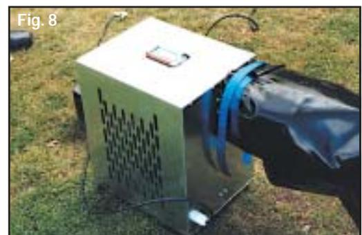
***It is vital to cover the fan if the weather is wet outdoors to avoid the fan shorting out. Also do not turn on its side as it may ingest grit or other material from the ground, which will damage it.***
