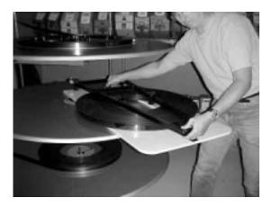
Roll the loaded transporter to the new location. Take care when rolling over any obstructions such as carpet edging or extension cords. The assembly must be carried over steps or large obstacles. Although the film roll cannot fall off, it may partially unravel or be damaged if the loaded transporter is handled roughly.
