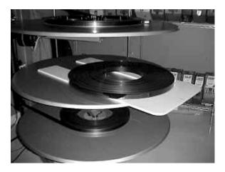
Lay the frame carefully onto the transporter plate and film. The film roll may need to be moved to allow the handscrews to align with the threaded inserts in the plate. Tighten all 5 handscrews finger tight, do not over-tighten.
