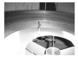
Guide the pin into the hole as you slide the transporter plate out. Once one pin is engaged, it is easy to align the second pin. Remove the plate entirely.
