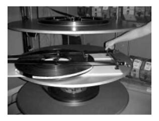
Grasp the upper frame rail and the lifting handle securely, and slide the assembly off the platter. Gently set the wheels down and tilt it to upright. Two people may be needed for this task.
