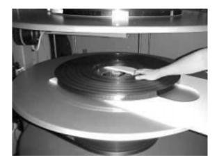
Centre the film pack on the transporter plate, with centre ring edge roughly at the curve of the notch in the plate.
