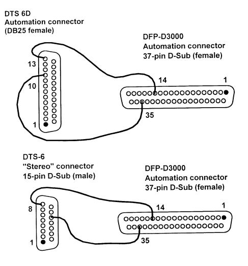
No DTS automation interface board is necessary. Please note that the DTS 6 system must be configured for 'CP200' by setting the two internal dip switches on the DTS output board to the "off" position by referring to the DTS 6 Installation Manual.
