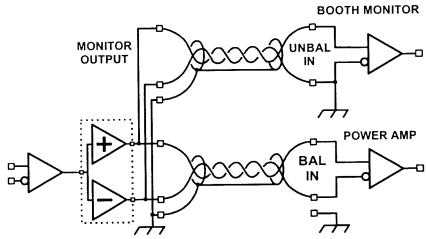
Notice that the unbalanced input of the booth monitor effectively unbalances the output of the DFP-D3000 as it connects its "cold" or out-of-phase side to the booth monitor's ground system. Nevertheless, if the wiring is done as illustrated, the power amplifiers will suffer no hum problems.
