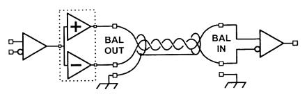
This circuit scheme gives the highest performance of all, because it offers the benefits of balanced outputs and the even greater benefits of balanced inputs. It is the approach taken in the design of Sony cinema processors at both their inputs and their outputs.
