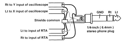
Use quality shielded cable and connect all the shields to the phone plug's sleeve common.
