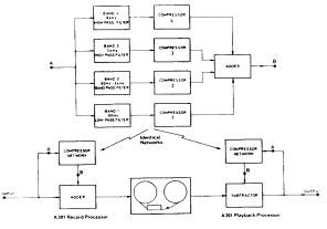
Noise Reduction System-Basic Block Diagram
