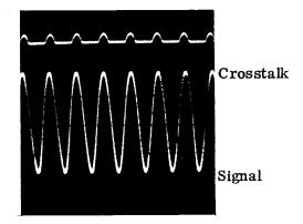
Oscilloscope traces of crosstalk. Upper trace, left channel; lower trace, right channel.
