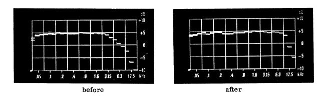
Fig. 7.6 Adjustment of Optical Pre-amplifier h.f. controls
