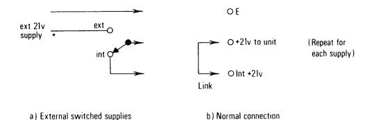
4. When the external power supplies are switched on, the unit should function normally. If not, check for possible damage to one or more of the modules due to power supply failure.
